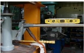
SHOWS HOLDING NACELL WHILE SETTING THE TAIL TUBE ANGLE.
