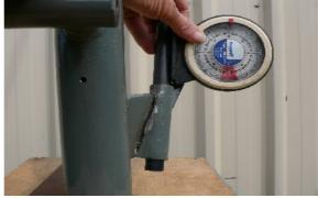
TOP LEFT - SHOWS SETTING SIDE ANGLE WITH AN INCLOMETER .
