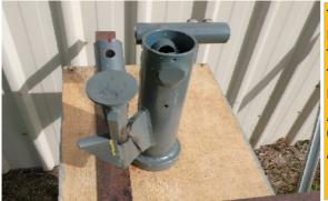
TO CHANGE THE ANGLES ( SIDE, BACK & BOTTOM STOP) IT IS BEST TO CUT JUST BEHIND THE WELD ON THE PIVOT BUSH, IT MAY BE BEST TO CUT IN FROM THE BOTTOM AND TOP LEAVING APPROX 10MM JOINED IN THE MIDDLE, THEN REMOVE MATERIAL FROM EITHER TOP OR BOTTOM OF THE CUT TO ALLOW THE NEW ANGLES.
