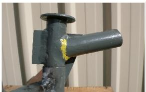
AFTER CHANGING THE TAIL PIVOT ANGLES THE TAIL SUPPORT TUBE MOUNT CAN BE ADJUSTED BY CAREFULLY CUTTING / GRINDING THE WELD AND RE- WELDING IT WITH A SLIGHT ANGLE UP.
