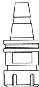
ISO-30 Tool Holders with covernut and pull stud for HSD Spindles
