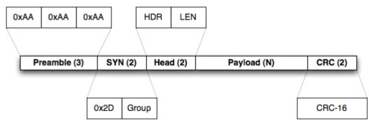
I made quite a few design decisions in the RF12 driver. One of the goals was to make the communication work in the background, so the driver is fully interrupt-driven. An important choice was to limit the packet size to 66 bytes of payload, to keep RAM use low and still allow just over 64 bytes of payload, enough to send data in 64-byte chunks with a *teeny* bit of additional info.
