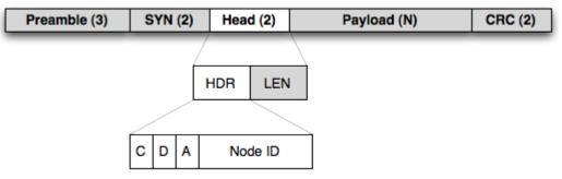
There are three bits: C = CTL, D = DST, and A = ACK, and there is a 5-bit node ID. Node ID 0 and 31 are special, so there can be 30 different nodes in the same net group.
