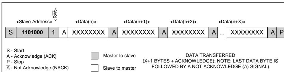
**Figure 6. Data Read (Write Pointer, Then Read)—Slave Receive and Transmit**
