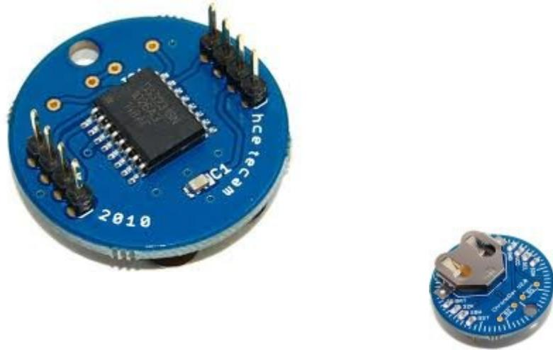
Love Electronics (UK) (DS3231S) +- 2 ppm (I used this device in testing)
