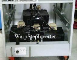
The actual final regulated output voltage can be readily potentiometer adjusted but we need a design goal to start from when designing our transformers initially.
