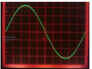
with every possible switching combination we can generate 3x3x3x3 = 81 possible voltage steps peak to peak. That is forty steps up, forty steps down, with a zero step in the middle.
