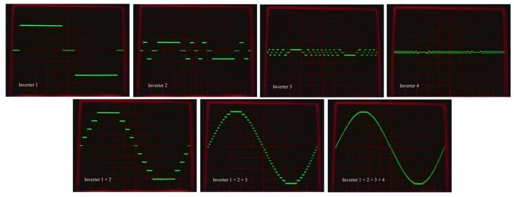
the the grid here. A four inverter stepped system with 81 steps peak to peak produces just slightly below 1% measured harmonic distortion without any filtering."
