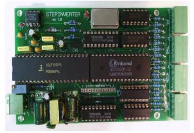
converter starts a conversion every 40mS and its output is latched into the rom every second cycle right at the zero crossing.
