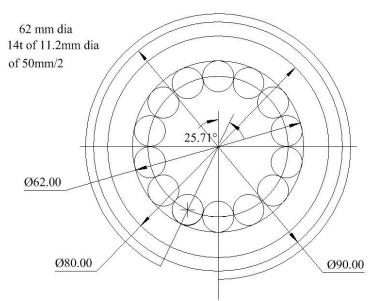
Here is a card template drawing with an original core hole
