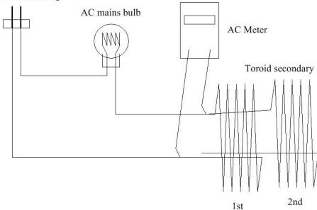
The secondary basic test circuit.
