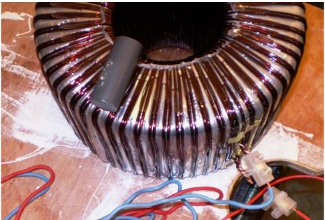
hot air and the tubing will shrink and the internal glue will melt.
