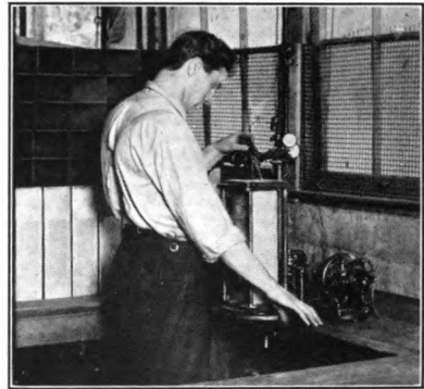
Making the Edison Container a one piece can by oxy-acetylene welding.
