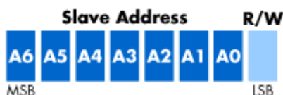
Figure 1: 7-bit addressing. The I2C bus specification specifies that in standard-mode I2C, the slave address is 7-bits long followed by the read/write bit.
