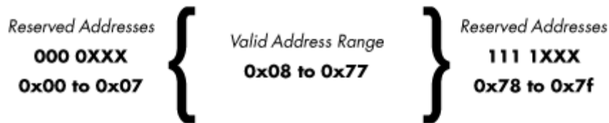
Figure 3: Valid 7-bit Slave Address Range. The range of valid 7-bit slave addresses are bound by two blocks of reserved addresses at either end of the range. Valid slave addresses are greater than 0x07 and less than 0x78.
